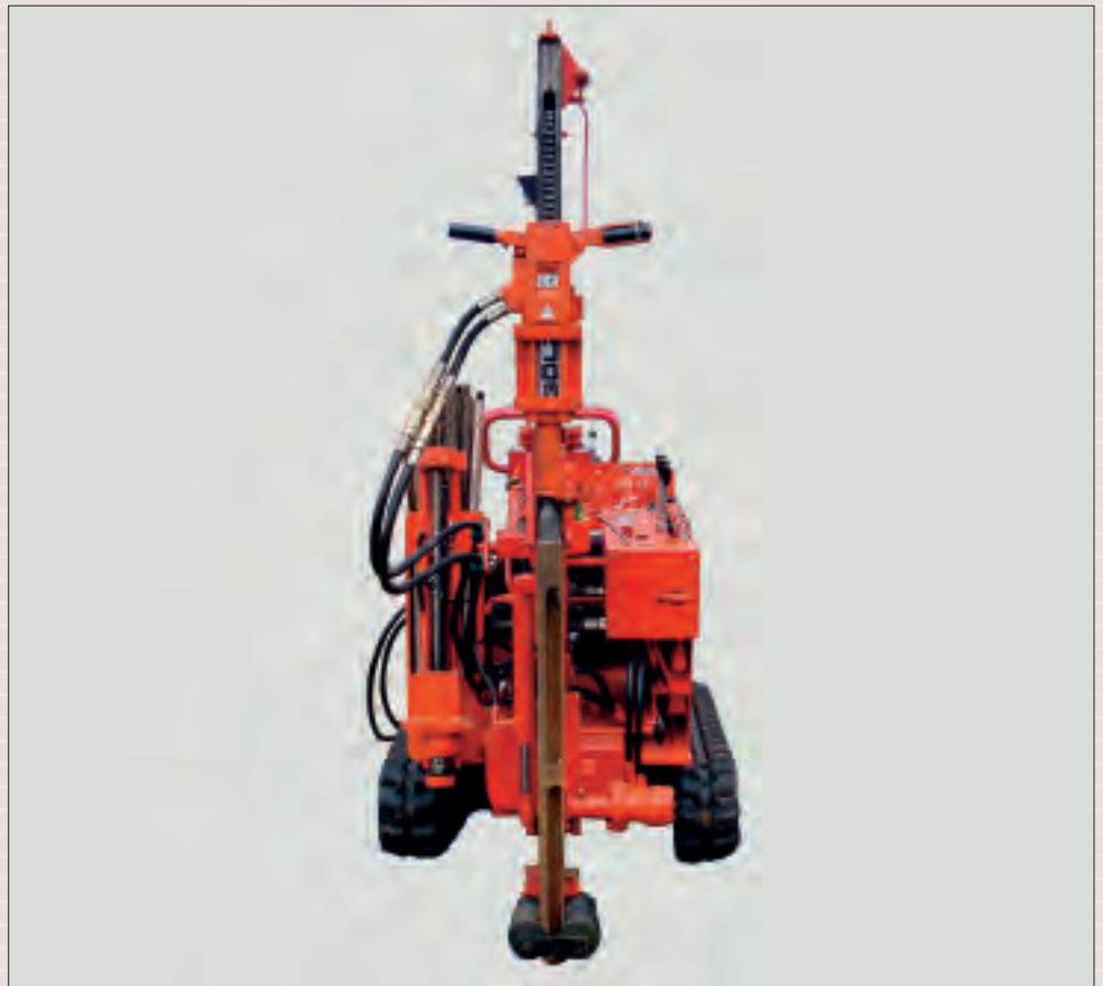
Fully hydraulic percussion drilling rig
